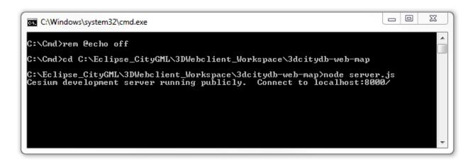
Fig. 5.1: Example of running the JavaScript-based web server
