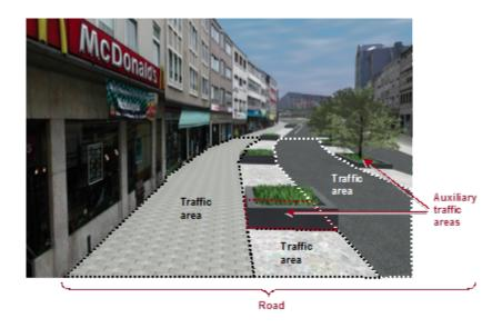
Fig. 2.18: LoD2 representation of a transportation complex (from: [GKCN2008])
