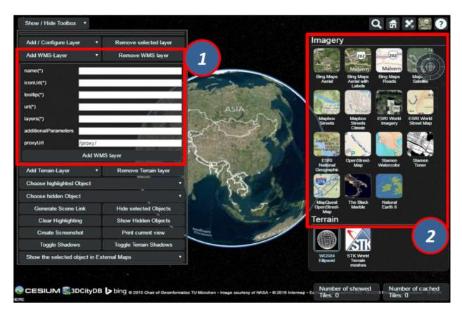
Fig. 5.14: The input panel [1] for adding a new WMS layer and the BaseLayerPicker widget [2] where the added WMS layers will be listed together with the per default available imagery layers
