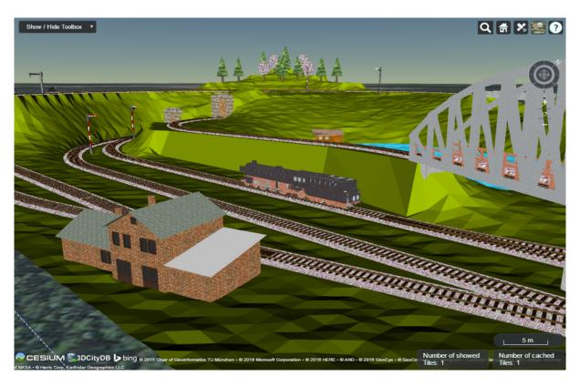
Fig. 5.34: Screenshot showing the example of displaying different CityGML top-level features (building, bridge, tunnel, water, vegetation, transportation etc.) in glTF format in the 3D web client
