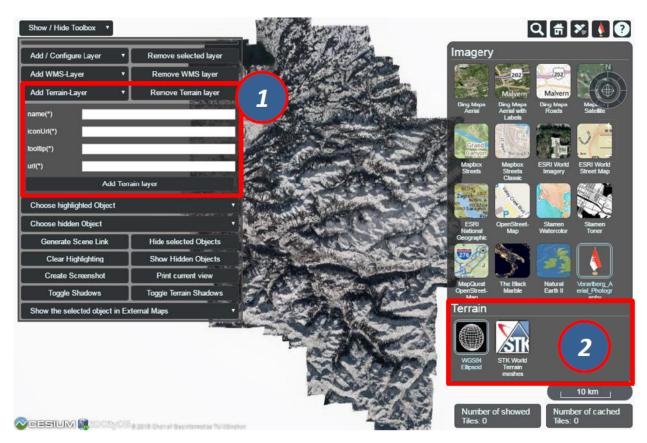
Fig. 5.16: The input panel [1] for adding a new terrain layer and the BaseLayerPicker widget [2] where the added terrain layers will be listed together with the per default available base layers
