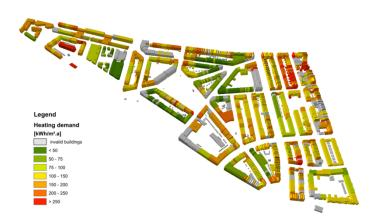
Fig. 6.3: Example of a 3D building heat demand map for the city of Ludwigsburg created with novaFACTORY 3D within project SimStadt
